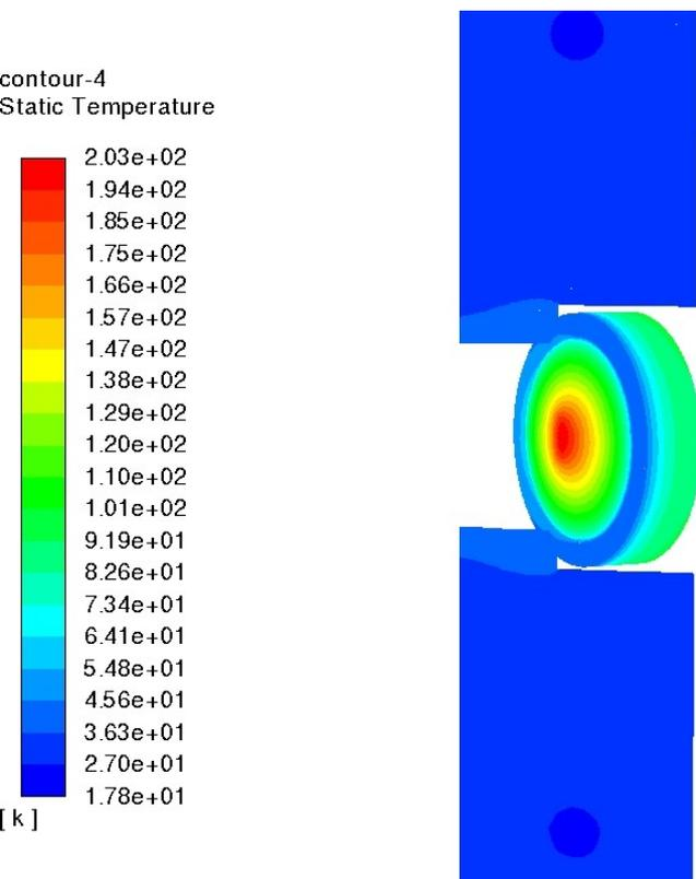
0.2 mm CaO film contact with the Cu frame, on one side of Ca,  $k_{\text{CaO}} = 5 \text{ W/m.K}$
