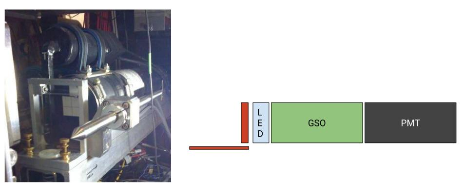
A metal cylinder is used to center (visually) the detector. It also provides a reference point for surveys. Due to interferences, it will be mounted only for installation.
