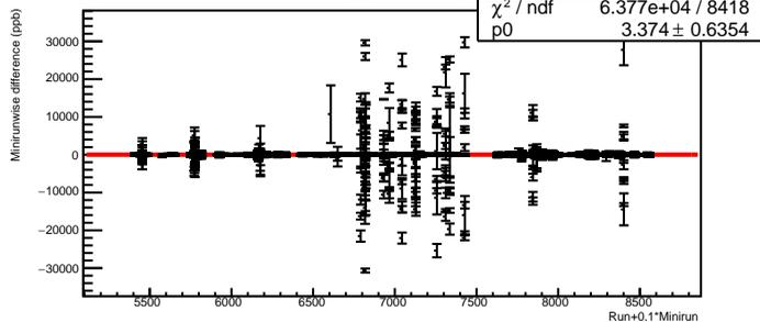
Minirunwise difference of regular dit vs. eigen dit, maindet weighted
