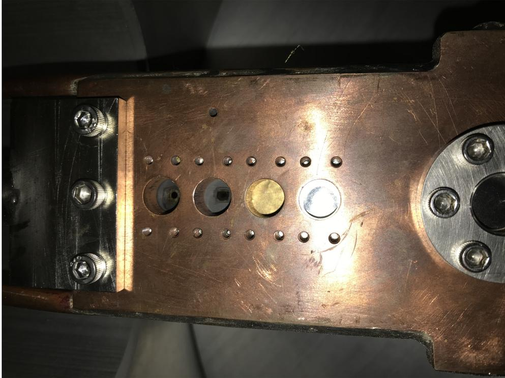
Figure 3: Water cooled prex2 target ladder configuration for summer 2019 run, upstream beam line view.
