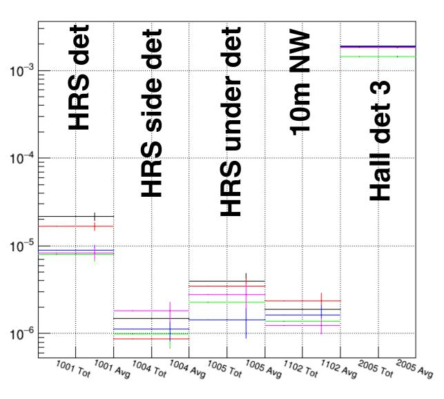
Black: current setup Red: current setup + 4 in donut Green: PREX 1 dump Blue: current setup + concrete Shield Magenta: current setup + Poly Shield
